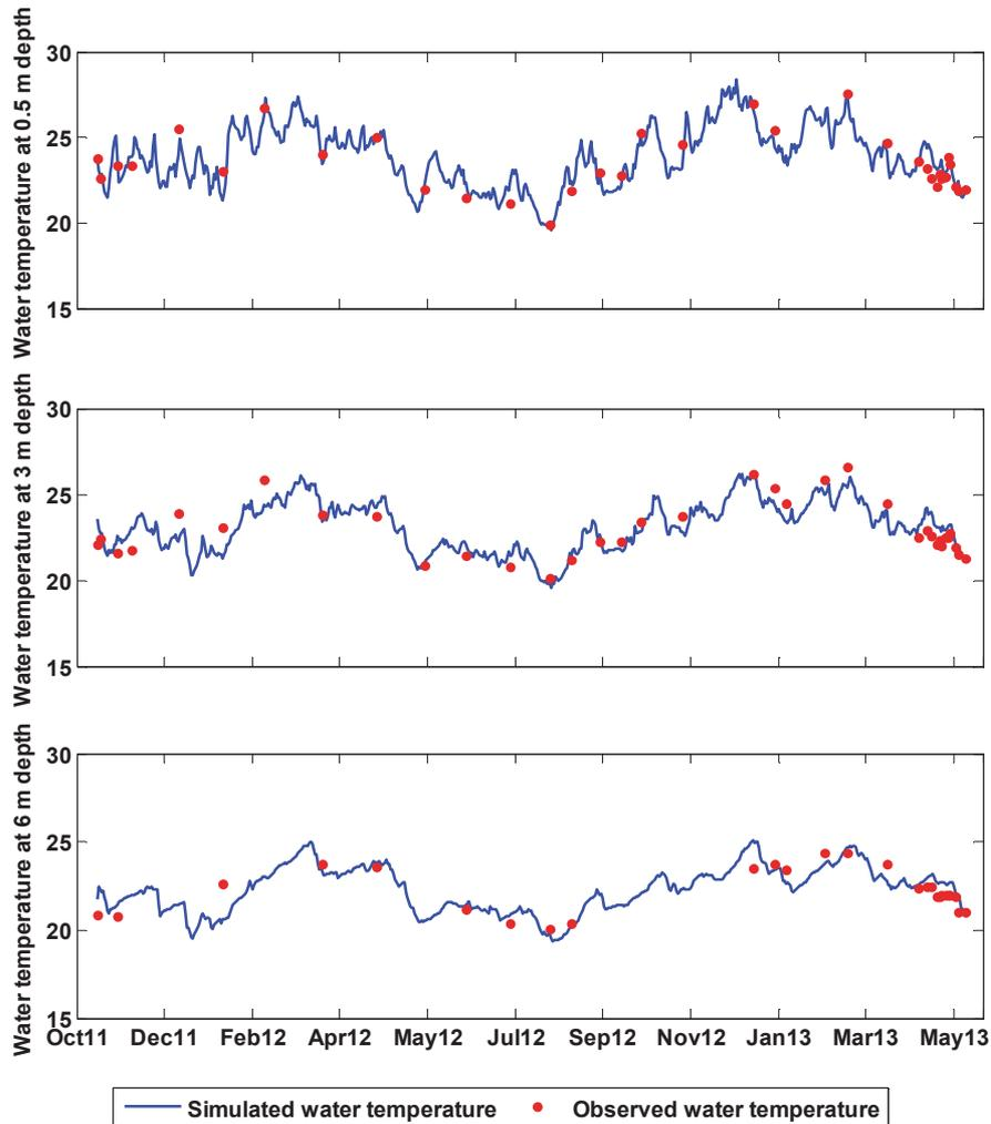
Figure 1 : Simulated (line) and observed (dots) water temperature in Lake Pampulha (point P1) at 0.5 m, 3.0 m and 6.0 m depth from October 18<sup>th</sup> 2011 to June 04<sup>th</sup> 2013.
