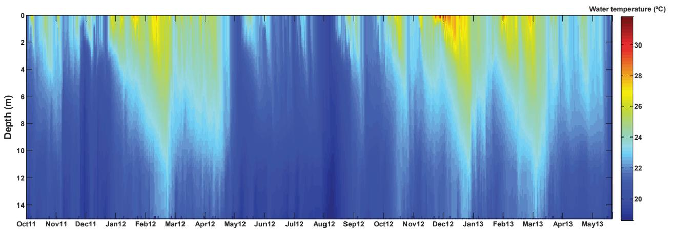
Figure 2 : Vertical variations of water temperature simulated by the GLM in Lake Pampulha (point P1) from October 18<sup>th</sup> 2011 to June 04<sup>th</sup> 2013.
