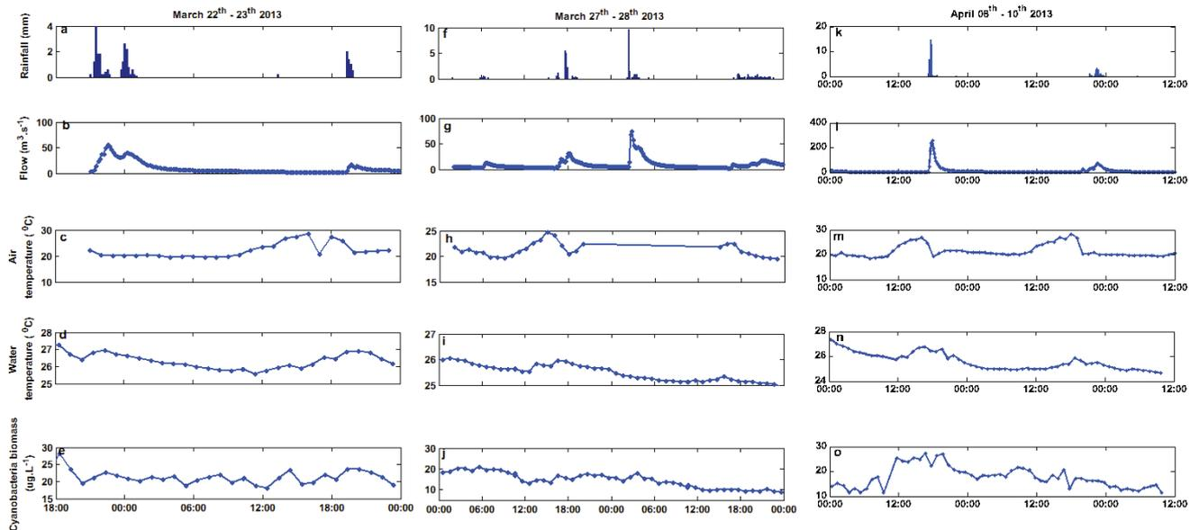
Figure 3: Stormwater runoff impacts on water temperature and cyanobacteria dynamics. a, f and k – Rainfall (mm); b, g and l – inflow into Lake Pampulha ( $\text{m}^3 \cdot \text{s}^{-1}$ ); c, h and m – Air temperature ( $^{\circ}\text{C}$ ); d, i and n – water temperature from SMATCH buoy ( $^{\circ}\text{C}$ ); e, j and o – cyanobacteria biomass ( $\mu\text{g chl-a} \cdot \text{L}^{-1}$ ).
